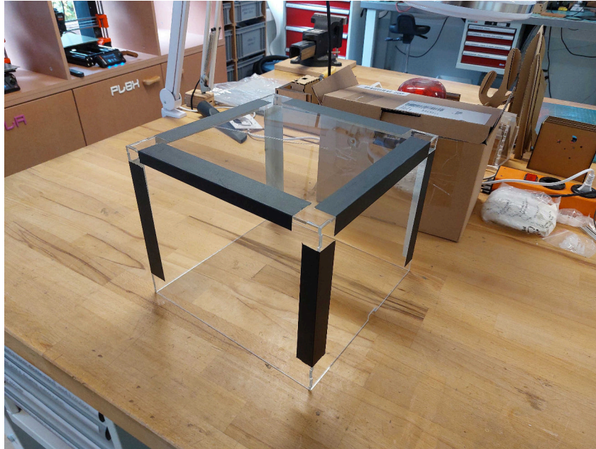
Figure 8: Test enclosure made out of laser-cut acrylic
